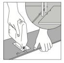
**7. Door molding and skirting:** Lay a board (with the decorative side down) next to the door molding and saw as shown in the figure. Then slide the floorboard under the molding.
